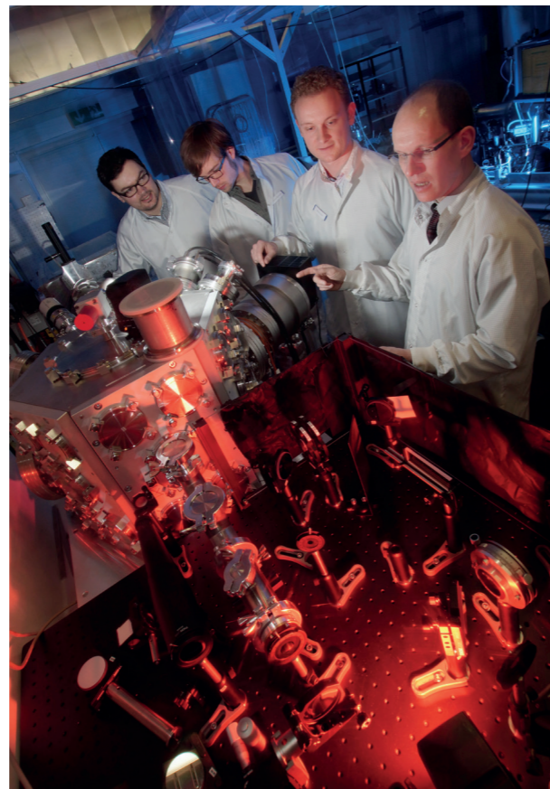
Extreme light-matter interaction experiments, for instance the access to ultrashort wavelengths, are performed by studies of femtosecond laser radiation in a vacuum or in a noble gas environment.
